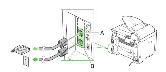
Connect your external telephone to the external device jack (A) on back side of the machine if required.
